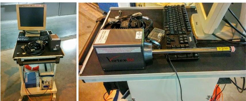
Left: view of the detector and readout electronics. Right: close-up of the detector
