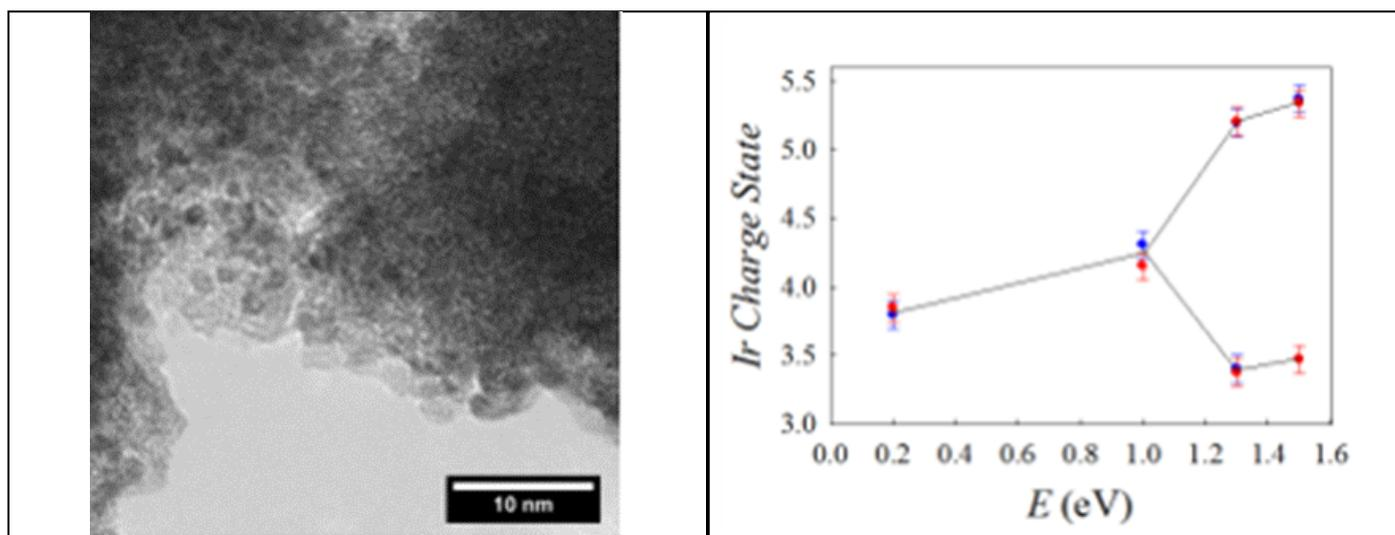
Figure 1, Left: an high resolution TEM image of the IrO<sub>2</sub>/Ir powder. Right: Dependence on the Ir charge state on the applied potential, obtained according to the Ir-LIII edge XANES peak thanks to the comparison with Ir(III) and Ir(IV) standards
