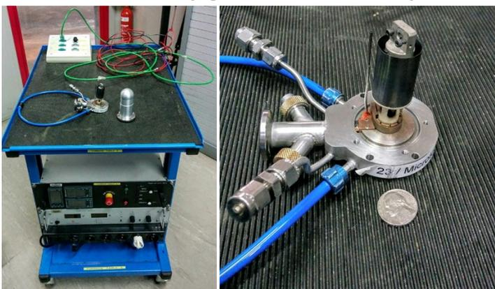
At the moment remote control is not possible and the target temperature needs to be entered manually, work is in progress to integrate the temperature control in SPEC. Test are also in progress to operate the microtomo together with a mass spectrometer for the analysis of the reaction gases.
