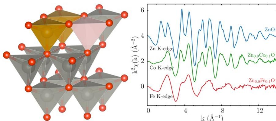
Figure 1, Left: Sketch of the ZnO structure (gray Zn and red O) with a hypothetical FeO<sub>4</sub> dimer (orange) coupled with a charge compensating Zn vacancy (pink). Right: comparison of the experimental Zn-, Co- and Fe- K-edge EXAFS spectra revealing oscillations of reduced amplitude at the Fe K-edge. This reduced amplitude is compatible with both the presence of cationic vacancies and/or the presence of interstitial oxygen.
