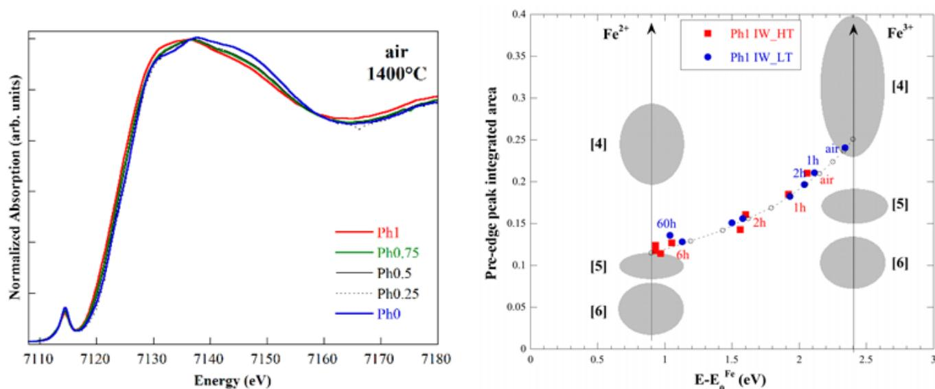
Figure 1, Left: XAS spectra of the five glasses synthesized in air at high temperature. In the edge region is evident a shift toward lower energies corresponding to the increase of the [Na/(Na+K)] ratio. Right: Plot of the pre-edge peak integrated area vs. centroid position for the kinetic experiments of glass Ph1 done at higher and lower temperatures (HT and LT, respectively). The evolution of the redox for different times is clearly different for the two different synthesis temperatures.
