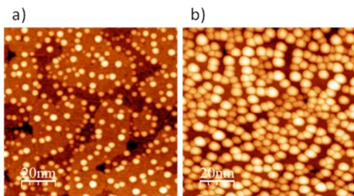
Fig. 1: STM images of Ag nanoparticles obtained by growing (a) 0.2 Å Ag and (b) 1.5 Å Ag on 10 ML thick (111) oriented CeO<sub>2</sub> films.
