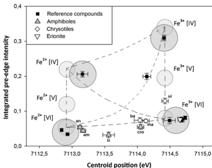
Figure 1: Pre-edge parameters of samples and reference compounds plotted in the modified variogram from [Wilke et al. 2005]. Little grey fields designate pre-edge parameters for the Fe coordination and oxidation state whereas dashed lines between fields indicate the variation of pre-edge parameters assuming binary mixtures of respective end-members. Darker grey fields designate our pre-edge parameter.
