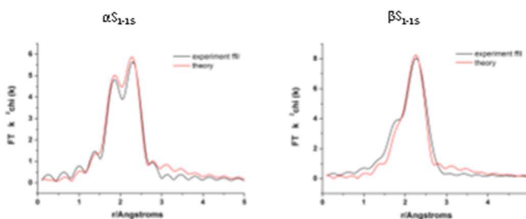
Figure 1, Comparison of the theoretical signal (red) with experimental data (black) of Fourier transforms of Cu K-edge XAS spectra of copper(I) complexes of  $\alpha$ S<sub>1-15</sub> and  $\beta$ S<sub>1-15</sub>.
