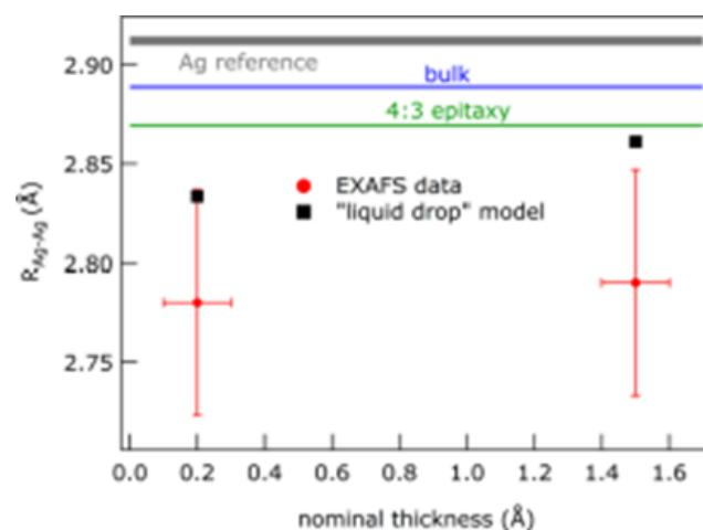
Fig. 2: Ag–Ag interatomic distance for the 0.2 Å Ag and 1.5 Å Ag samples on CeO<sub>2</sub> obtained from the EXAFS analysis. The thick grey line is the value measured on the metallic reference sample. The green line is the value expected assuming an epitaxial contraction of 0.7%. The black squares represent the values obtained for the dimensionality-related contraction using the “liquid drop” model.
